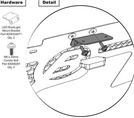
This is the recommended time to install your LED Rock-lights and wiring onto the vehicle and wheel well liners, per best practices and per the lighting manufactures in-structions.
