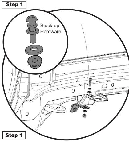
Stack-up the M6 Bolt (3000722), with Lockwasher (3000136), and Flatwasher (30).00288
