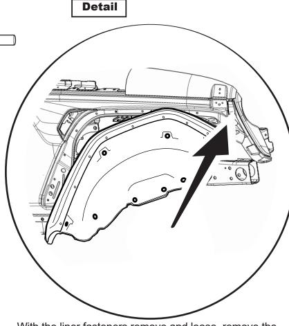
With the liner fasteners remove and loose, remove the entire fender. Firmly grasp inner fender and pull from body.
