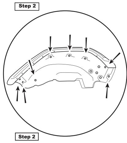
Next, releasing the inner fender liner push-in retainers. Pry all the plastic trees that join the liner to the Jeep body.
