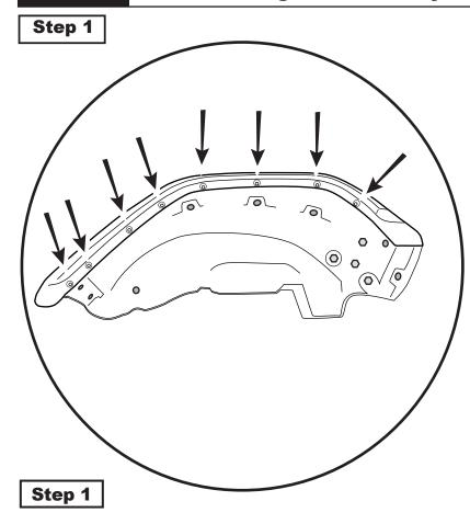
On the OEM front fenders. It may be easier to cut the head off the 8 retainers with cutters.
