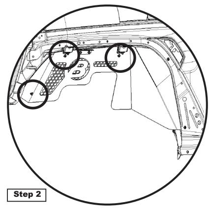
Install Fender Liner to the previously adjusted hanger brackets in the four locations as shown above. Install M6 Combo Bolts (3006267). Do not install any additional hardware.
