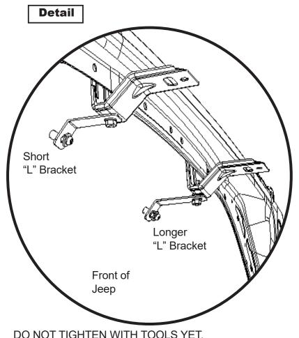
You will need to have the fenders loose incase of needed adjustments in final steps.
