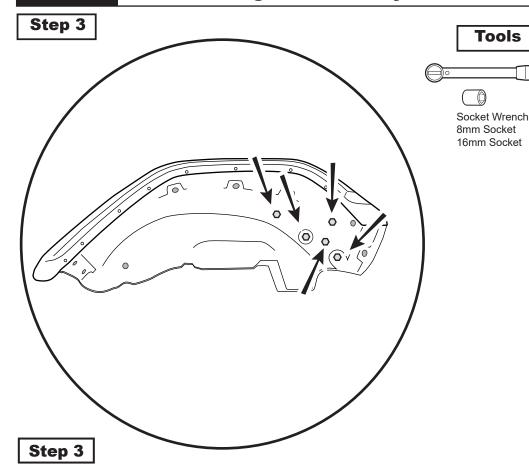
Now remove the last inner bolts that are holding the splash shield to the DRL fender light. There are five (5) bolts to remove,
